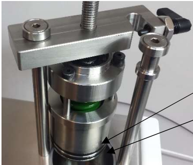
Second black O-Ring First black sealing O- Ring
